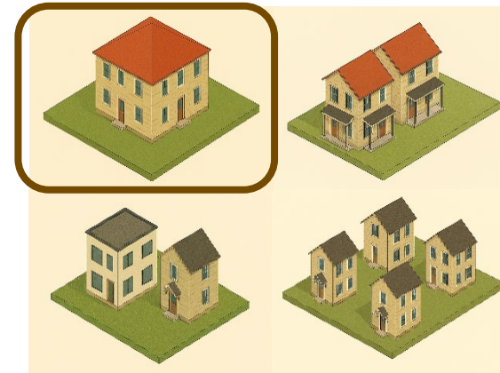
Various configurations of 4 attached and detached units. The upper left is a fourplex, while the other configurations are "multi-dwelling development."
